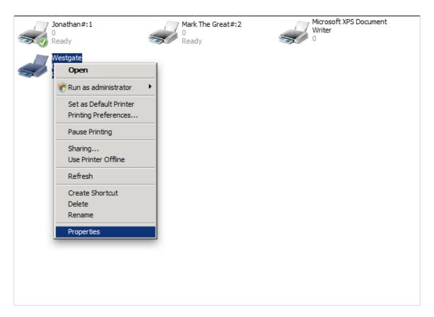
4. Select the **Device Settings** tab. In this list of options there should be a setting for whether or not the printer has a duplexer installed. Switch this from uninstalled to installed. Click **Apply** and then **OK**.
